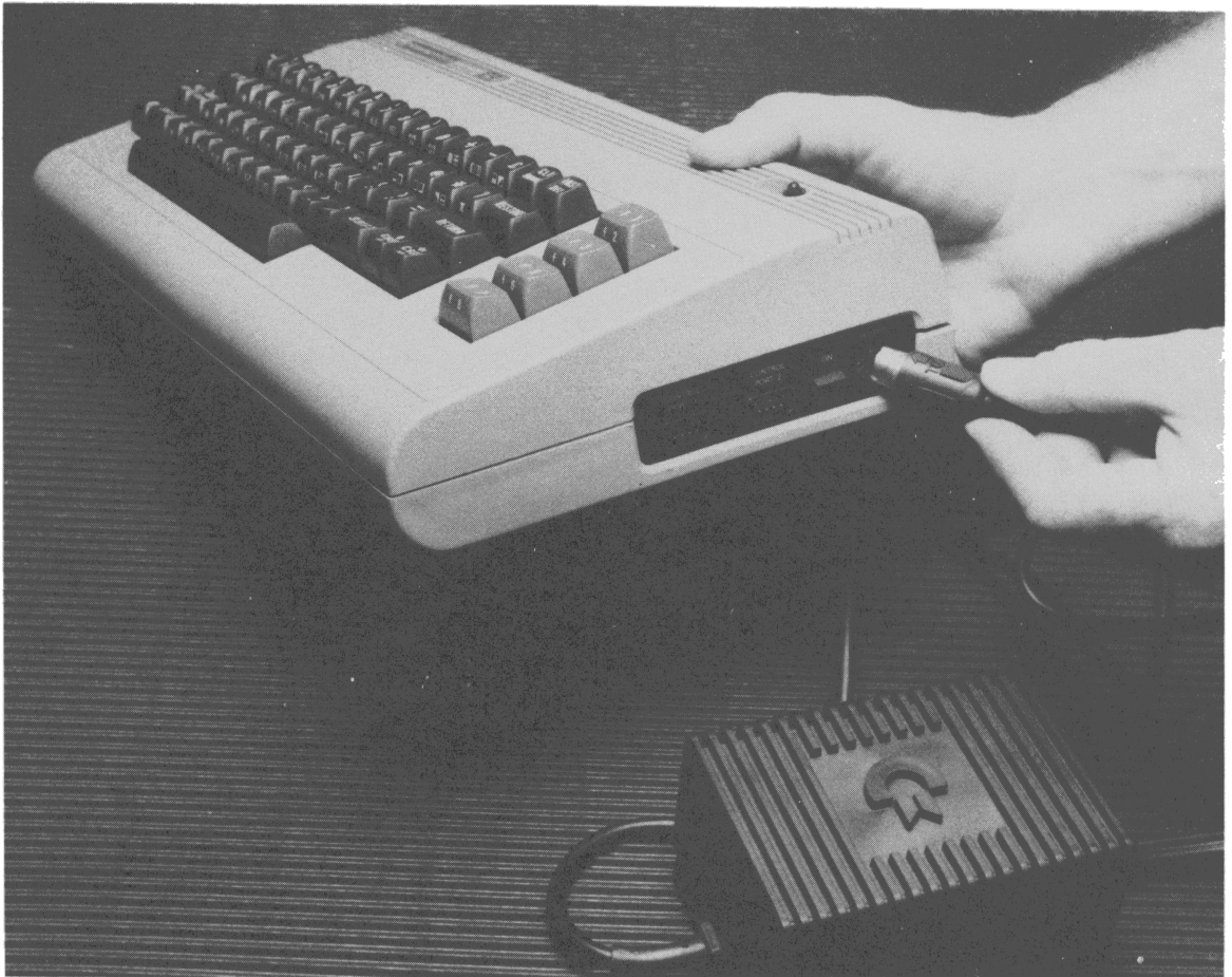
Fig. 1-2. The first obvious step to take when your 64 acts dead is to make sure it is plugged in at the wall socket and at the side of the case.
