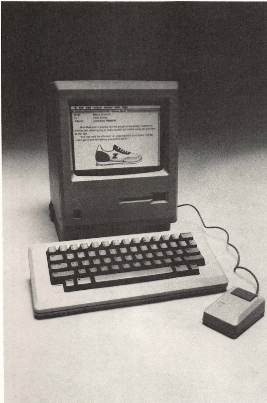
Fig. 1-2. Apple Computer's new Macintosh: extraordinary computing power and exceptional ease of use. Macintosh's main unit, which weighs less than 17 pounds, contains a 32-bit microprocessor, a built-in 3½-inch disk drive, a 9-inch black-on-white display, 64K of ROM and 128K of RAM. Equipped with a detachable keyboard and a mouse pointing device, Macintosh fits quickly and easily into the work style of business people, professionals, and students. The suggested retail price for Macintosh is only $2,495. (Courtesy of Apple Computer, Inc.)
