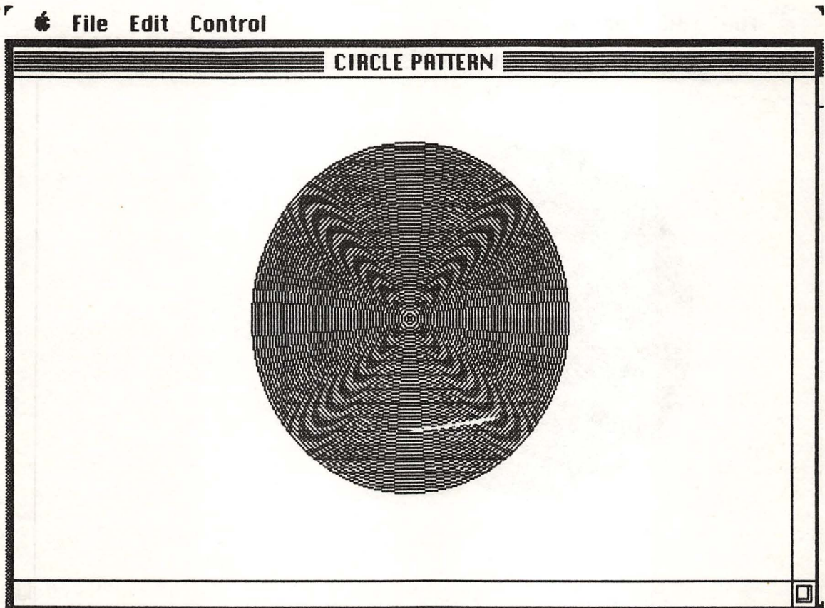
Fig. 10-6. A circle pattern created using a FOR-NEXT loop and the CIRCLE command.
