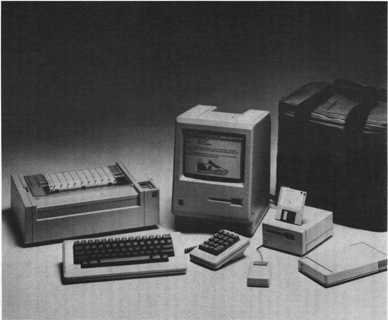
Fig. 1-1. Apple Computer's Macintosh is shown here with mouse and detachable keyboard. Peripheral devices and accessories include a numeric keypad, an external disk drive, the ImageWriter printer, a modem, and the Macintosh carrying case. (Courtesy of Apple Computer, Inc.)
