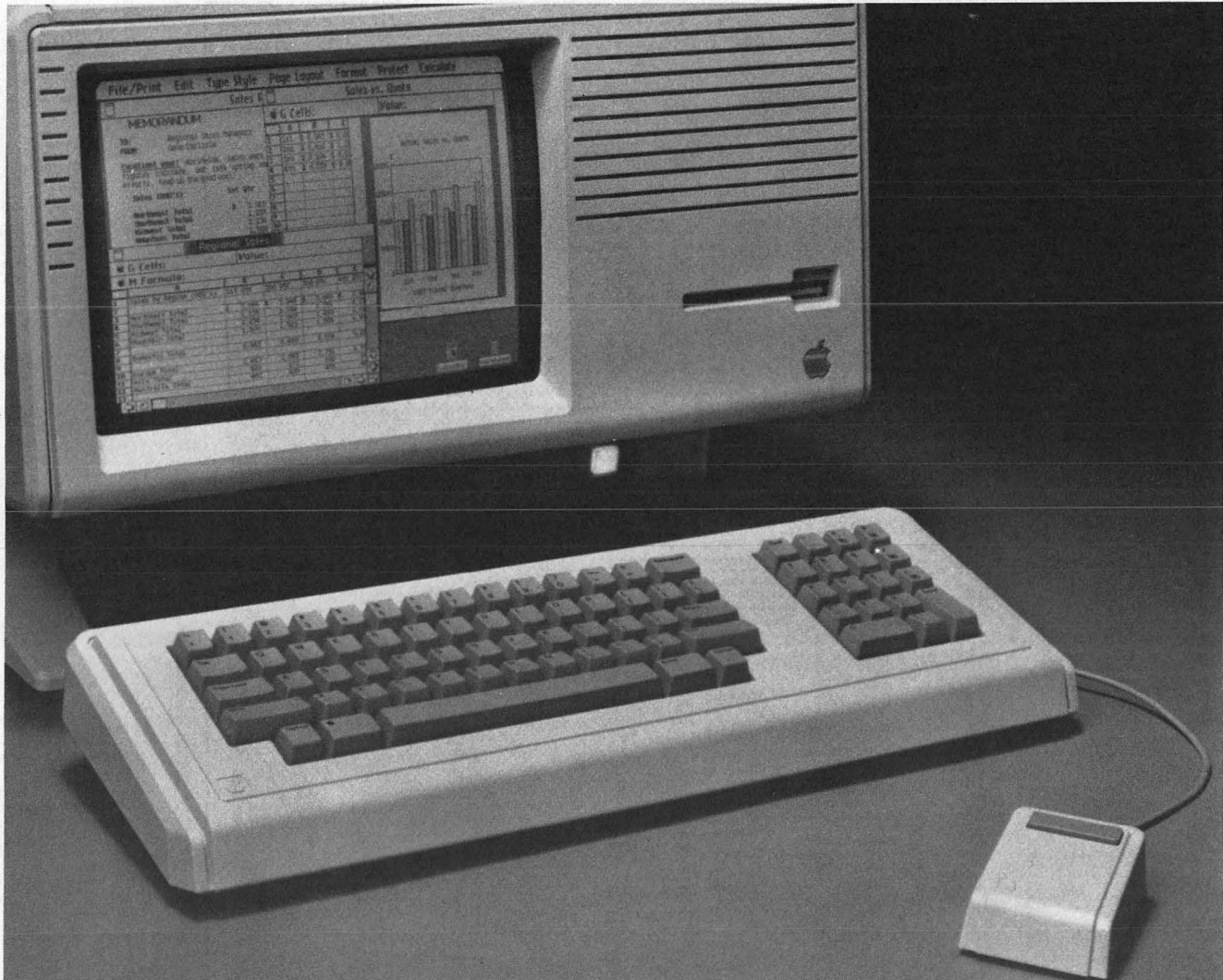
Fig. 1-10. Three new Lisa (TM) personal computers were introduced by Apple Computer, Inc. in January 1984. All three systems share the same look and feature advanced microdisk technology. The Lisa 2, the Lisa 2/5, and the Lisa 2/10 all have 512 kilobytes of internal memory, expandable to one megabyte. In addition, the Lisa 2/5 has a 5-megabyte external hard disk drive and the Lisa 2/10 features a built-in 10-megabyte hard disk drive. (Courtesy of Apple Computer, Inc.)
