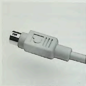
Figure 3-2 The 8-pin, minicircular connector
