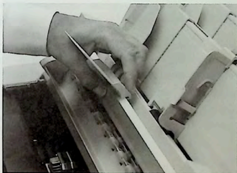
Figure A-19 Attaching the paper deflector
